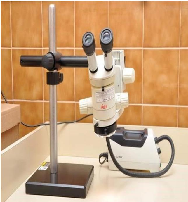
LUPA BINOCULAR ESTEREOSCÓPICA PARA PIEZAS MACROSCÓPICAS.
